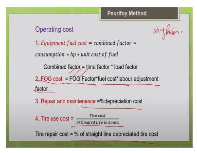
Now coming to the operating cost so equipment fuel cost so you can calculate it based upon the fuel consumption. So this fuel consumption you can get it from your past record or any equipment handbook or the manufacture guideline. So which ever manufacture supply the equipment so they will be provided some guidelines of the handbook in the handbook you can get your information for a particular model on the hourly fuel consumption.
